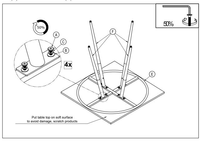
**STEP 2**: ATTACH CROSSBAR (G) TO LEG OF TABLE (F) (H) WITH BOLTS (A), WASHER (B), SPRING WASHER (C) USING ALLEN KEY (D). DO NOT TIGHTEN COMPLETELY.
