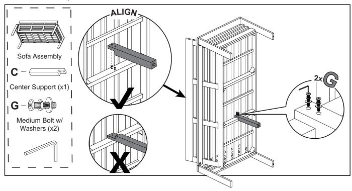
STEP 8: **ALIGN** the second Center Support (C)x1 over the opposite Seat Support so the bolt holes are aligned with the threaded inserts and the notch sits beneath the Seat Support, as shown. Then **FASTEN** with Medium Bolts w/ Washers (G)x2 through the Center Support (C)x1 into the threaded inserts in the Seat Support as shown. First tighten both <u>by hand</u>, then complete with the provided Allen Wrench.
