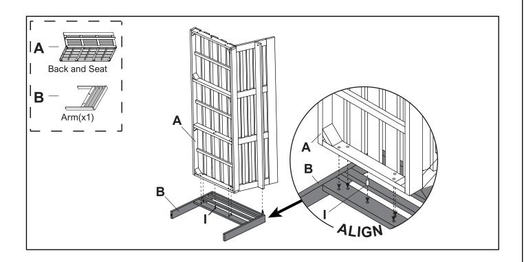
STEP 4: **FASTEN** Back and Seat (A) to the Arm (B)(x1) with Long Bolts w/ Washers (F) x4 and Short Bolt w/ washers (H)x1 first <u>by hand</u>, then tightening with the provided Allen Wrench, as shown below.
