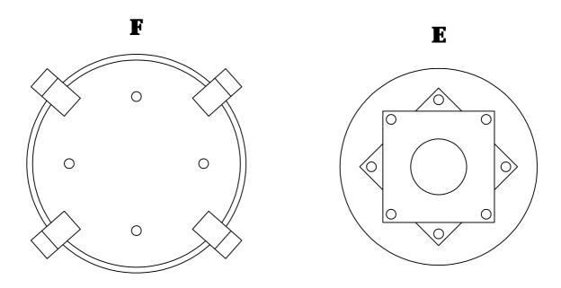
STEP 2: Using the bolts ,lock washer and flat washer to connect top seat and base frame, until tight and secure. Repeat for all other holes
