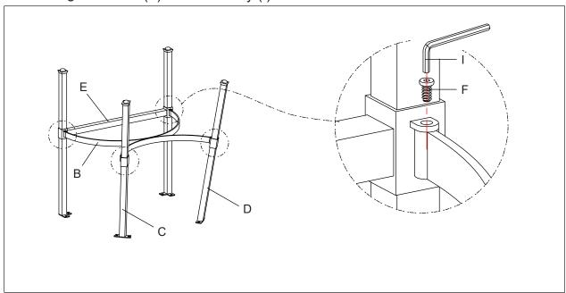
**STEP 2:** Assemble Seat (A) to the Legs using Allen Bolts (G), Flat Washer (H) and Allen Key (I).
