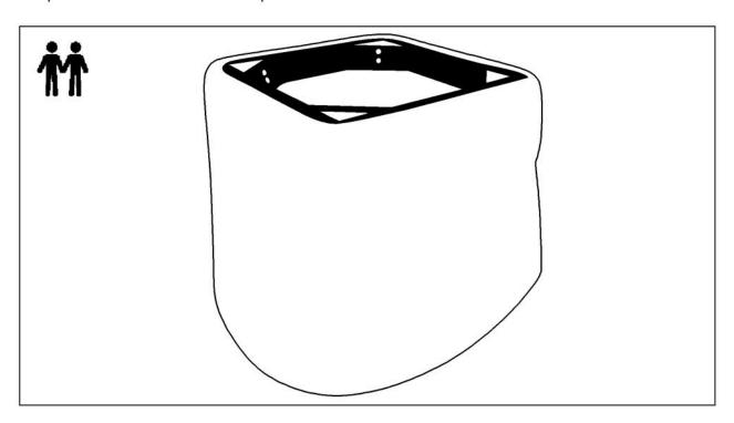
STEP 2: Align the back legs with bottom hole and tighten the screws clock wise with help of allen key.
