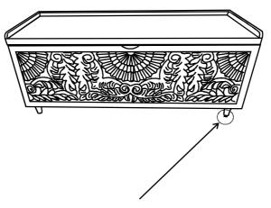
NOTE: Levelers can be used for adjustment if needed.
